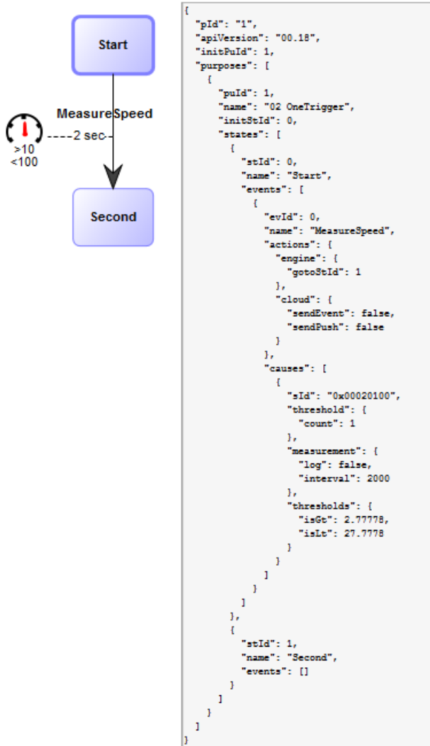
Figure 3. Test model for measuring speed
